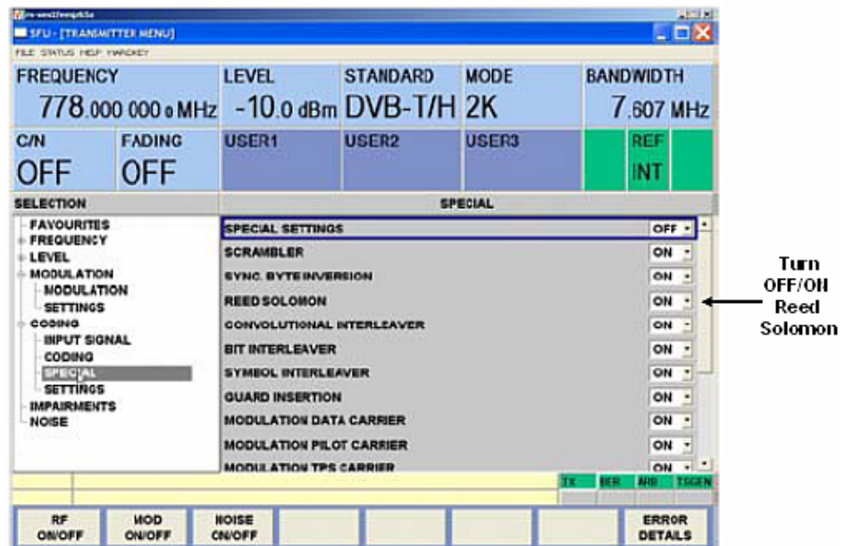
Figure 7 The Reed Solomon encoder on the R&S® SFU can be enabled/disabled.
